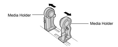
**4.** Place a media roll between the Media Holders so that the media is fed with the print side facing up. Fit the projection of the Media Holders into the core. Make sure that the projection of the both Media Holders is engaged with the core firmly.
